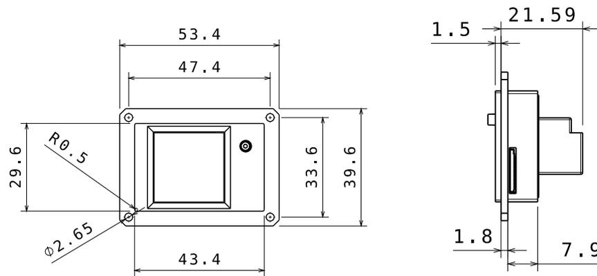
Figure 4-11: Display unit E1 (front view / side view)
