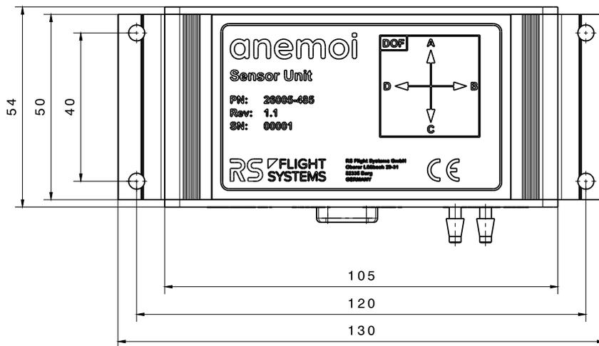
Figure 4-14: Sensor unit (top view)
