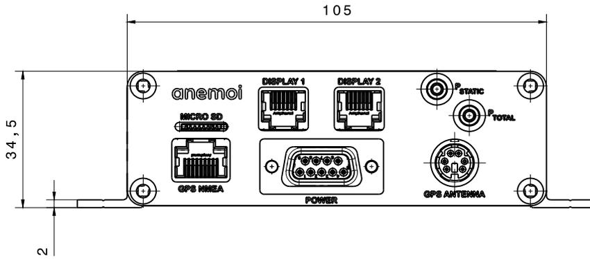
Figure 4-13: Sensor unit (front view)
