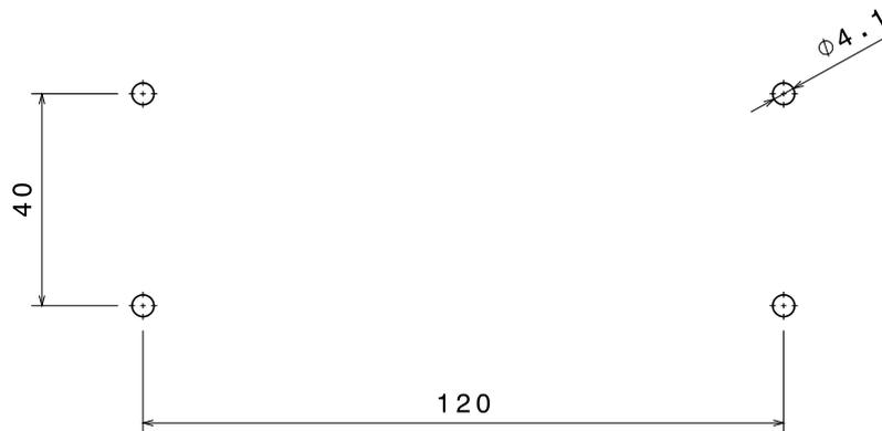
**Figure 4-5: Mounting cutout sensor unit**
