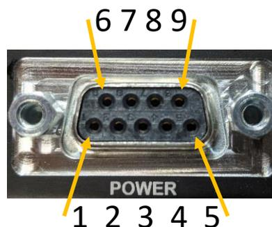
Figure 5-4: Power Connector pin allocation (D-Sub standard)
