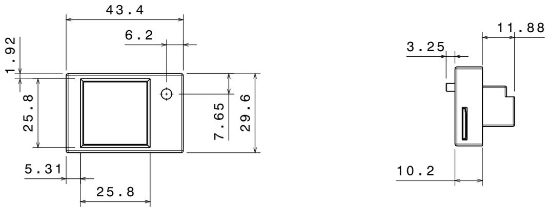
Figure 4-8: Display unit (front view / side view)
