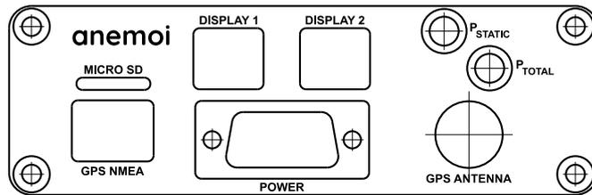
**Figure 5-1: Sensor Unit Front View**
