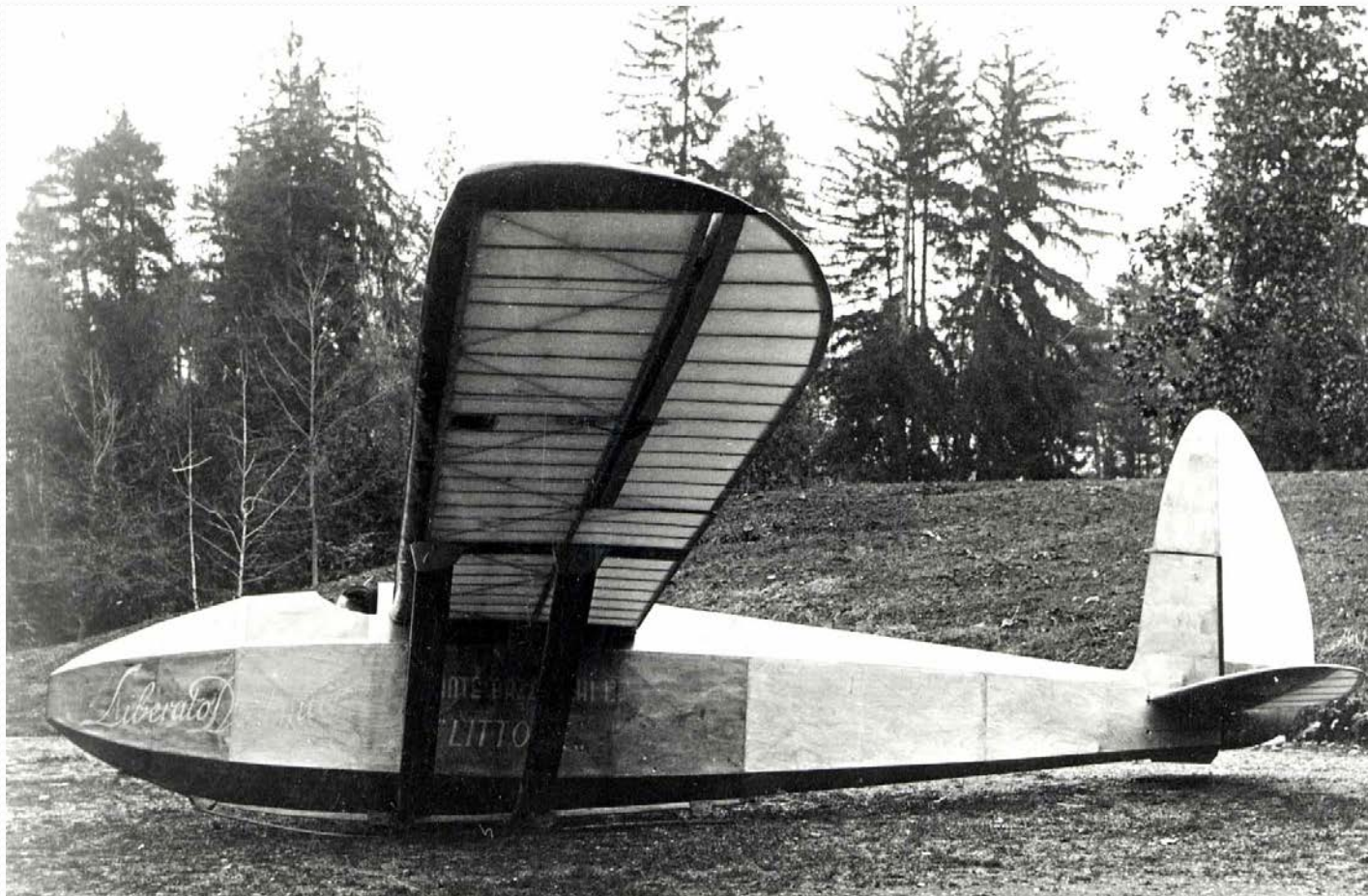
The EB-1 glider featuring a faired cockpit and properly shaped bracing attachments.
