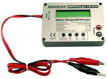
displaying the amp-hours it's sent to the battery, a useful indicator for verifying proper charging.
