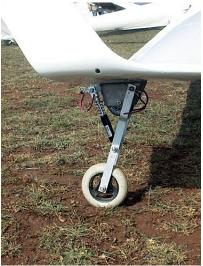
Taxiing on rough or soft ground may not be practical with the usual small wing tip wheels. Using a larger temporary tip wheel can save the day, though it must be removed before flight. DG Sailplanes makes one that can be folded and stowed in the baggage area after removal.
