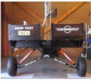
The patented ALG landing gear had to go through several tests for the certification process (FAA-EASA)
