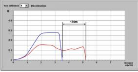
Nota: BERINGER brake pads used int the ALIR system have a friction coefficient that increases with the temperature allowing an increase of the deceleration when the lift decreases on the wings. Gear Wheels Brakes Nose wheel Tailwheel
